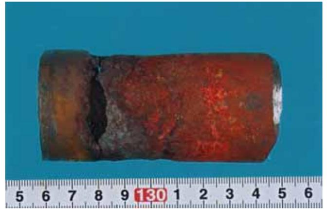
Thinned tube by the corrosion
