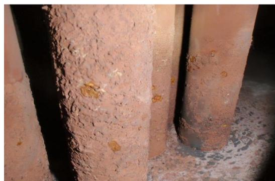
Corrosion by blow-off shortage
